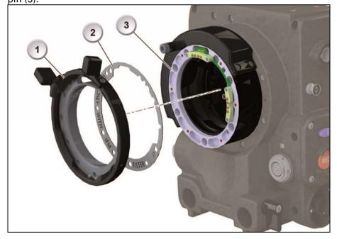
9. Fasten the lens lock, still in position OPEN (2), back to the PL mount; use two of the six torx screws (1) hand-tight:
