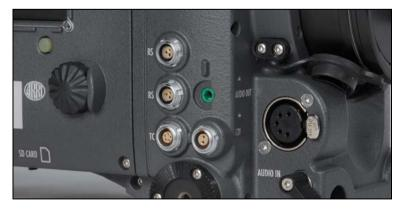
Figure 31: Connectors on right side
