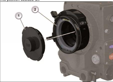
2. Unscrew (only with a TX6 torx screwdriver!) the four accessible torx screws (1) that hold the lens lock (the other two torx screws are still hidden by lock position CLOSED).
