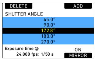
Note: When mirror shutter is active, the shutter angle is limited to 180.0 degrees. Frame rates higher than 37 fps for 4:3 and higher than 48 fps for 16:9 reduce the shutter angle range further.
