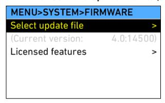
To keep the ALEXA up to date with new features, the camera firmware can be updated by the user. Download the latest Software Update Packet (SUP) from http://www.arri.com/camera/digital\_cameras and be sure to read the included instructions.
