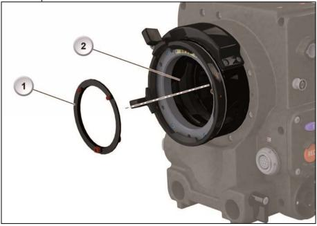
5. Screw the IFM-1 Reflex Tube into the PL mount, using your fingers. Do not touch the delicate sensor glass.
