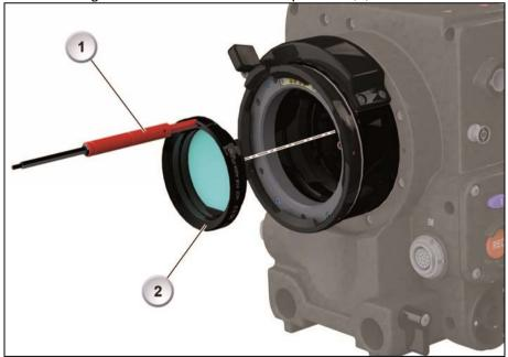
7. Place the next filter onto the bottom ring in the camera's PL mount. The Ground Glass/Frameglow tool has to be in the 12 o'clock
