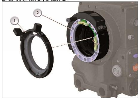
5. Remove the LDS pin support and MCA print (2) by unscrewing the four TX6 torx screws (1).
