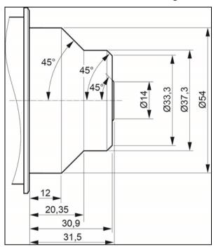
Figure 134: Allowed lens dimensions with in-camera filters
