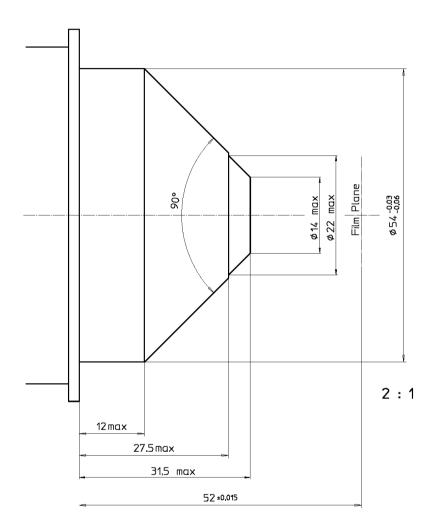
Figure 99: Allowed lens dimensions with mirror shutter
