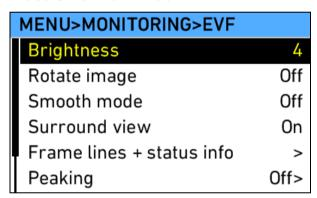
Brightness Select to adjust the brightness of the EVF.
