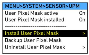
All sensors exhibit a certain number of defect pixels, and ALEXAs have two mechanisms to catch and correct them: one is a static pixel correction based on a pixel mask created during manufacturing, and the other is a dynamic pixel correction that continuously evaluates each frame and masks defect pixels that are not caught by the static pixel mask. In very few cases we have observed some pixels that are not corrected by either method; for those cases we have developed User Pixel Masking.
