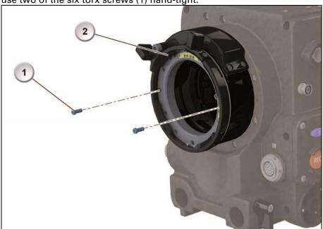
Turn the lens lock into Position CLOSED (2) and fasten the other four torx screws hand-tight (1). Check if all screws and the shim fit correctly:
