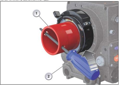
4. Accurately insert the IFM-1 Bottom Ring (1) into the PL mount (2). The square red nut must be in the 6 o'clock position and face camera-outwards, with the two smaller red pins taking the 10:30 and 1:30 positions.
