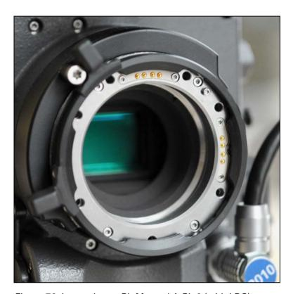
Figure 76: Lens adapter PL-Mount LA-PL-2 (with LDS)
