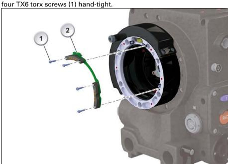
8. Accurately place the IFM Shim, with its inscription always facing camera-outwards (2), onto the PL mount. The shim's screw holes must line up exactly with the mount's thread holes and the index pin (3):
