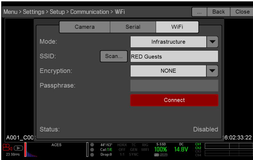
10. Connect your device to the same wireless network that the camera is connected to. The steps in this procedure depend on what type of device and operating system you are using. For example, if you are connecting an iOS device, go to **Settings > Wi-Fi**, and select the wireless network.
