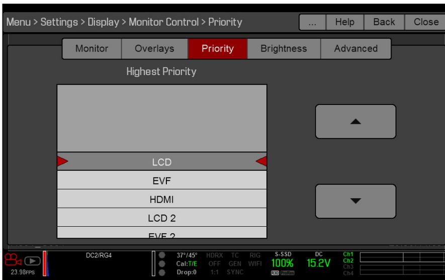
The camera can only have one (1) control monitor for interacting with camera settings. The Priority tab determines the order in which a monitor becomes the control monitor. If you plan on removing or adding monitors during a shoot, set up the priority list ahead of time.
